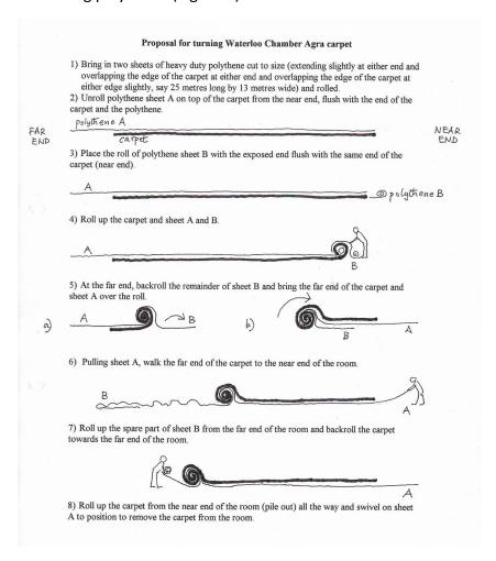
Figure 1. Diagram of rolling procedures used in 1998 ©Jonathan Tetley
