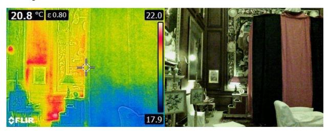
Figure 9 (left) and 10 (right). Thermal image of the back wall in the 2nd George room with the corridor running behind, with corresponding image, highlighting heat spots © The Landi Company
