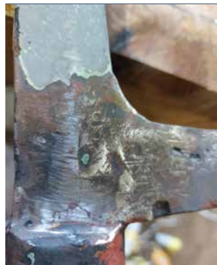
Above: The outer frames all contained a distinctive and unusual fire weld
