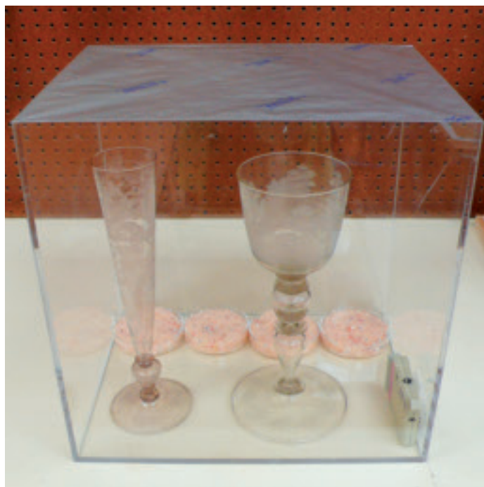
Perspex container sealed with Marvelseal and double sided tape
