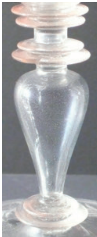
Loss and crystals inside stem
