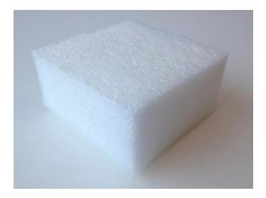
Ethafoam 220 appears very similar to PolyPlank EXT220 and PolyPlank LAM220, another brand name of polyethylene foam, but the two PE foams are manufactured with slightly different methods and chemical compositions. PolyPlank has a larger cell structure on average, and the broken cell walls of cut surfaces feel rougher. It offers less resistance to compression and puncturing than Ethafoam of the same weight. PolyPlank LAM offers two more light-density options than Ethafoam; 0.9 pcf and 1.2 pcf.
