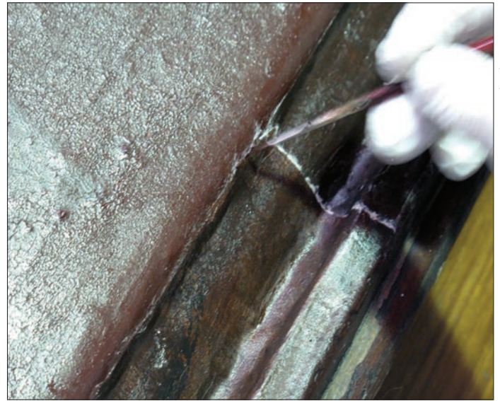
Colour matching Japanese tissue paper to the colour of the original vehicle roof guttering
