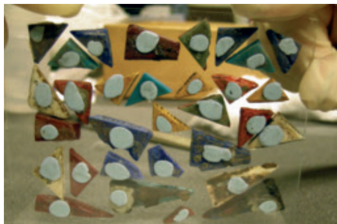
Fig 1 Blu-Tack holding objects to mount
