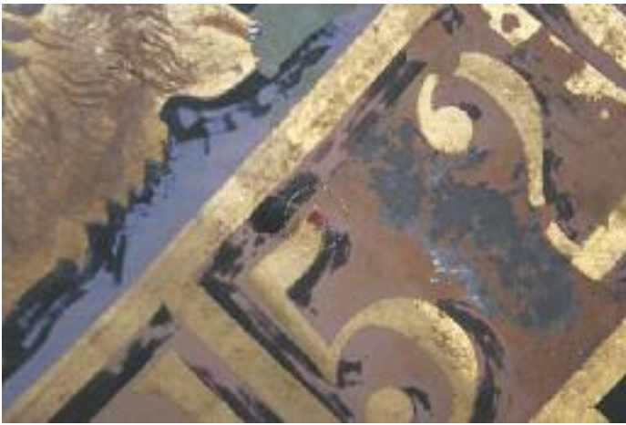
Figure 5 An area of unfaded red paint is uncovered below the gilding on the Sidereal dial. To the right the paint has been lost entirely and the lead-tin coating can be seen. (Photograph courtesy of Granville & Burbidge)
