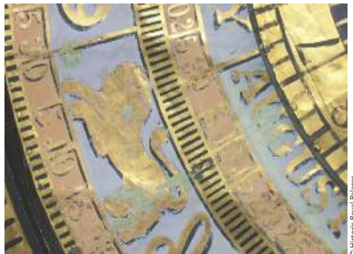
Figure 4: Detail of the condition of the painted surface on the sidereal dial before treatment. The green areas are where the undercoat is showing through.
