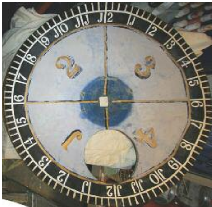
Figure 9 Lunar dial before cleaning. Note the chalkiness of the blue paint in comparison to the part that has been covered by the central world disc.
