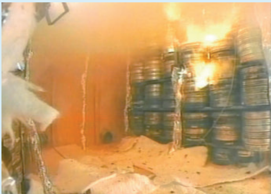
Stills from an Imperial War Museum film showing the test run of a nitrate film cell. Nitrate film is almost impossible to extinguish if it catches fire. IWM researched and trialled the use of individual film cells that vent out any fire (below) to prevent it spreading to adjoining cells. IWM now has a full facility of these environmentally controlled cells in Cambridgeshire.
