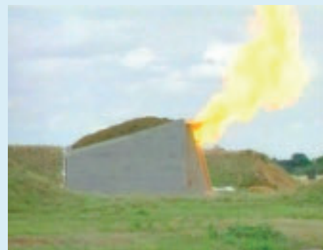
Stills from an Imperial War Museum film showing the test run of a nitrate film cell. Nitrate film is almost impossible to extinguish if it catches fire. IWM researched and trialled the use of individual film cells that vent out any fire (below) to prevent it spreading to adjoining cells. IWM now has a full facility of these environmentally controlled cells in Cambridgeshire.
