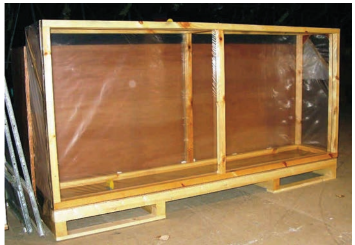
The prototype bubble crate, with the five-sided wooden crate behind it
