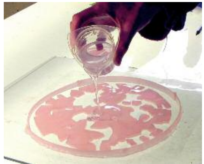
Pouring Araldite 2020® into mould
