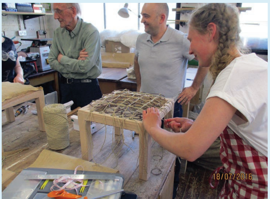
Hannah tying down the springs
