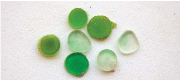
Orasol dyes premixed in acetone before being added to HXTAL NYL-1
