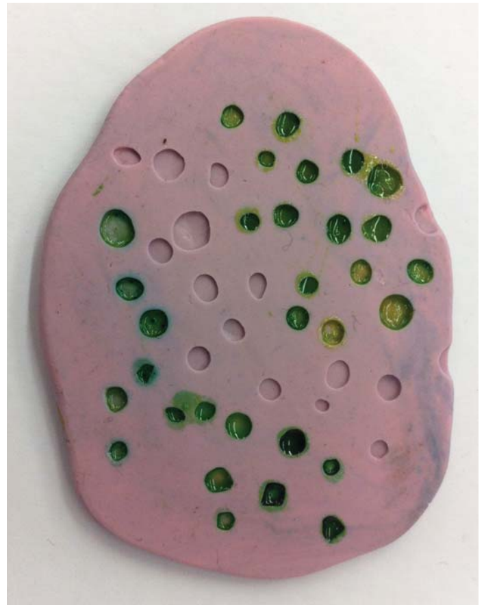
An impression was taken of the 'scales' using Lab-Sil silicone putty to make a mould
