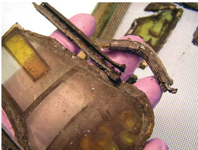
The cement after exposure to the DCM vapour, now pulled away from the glass
