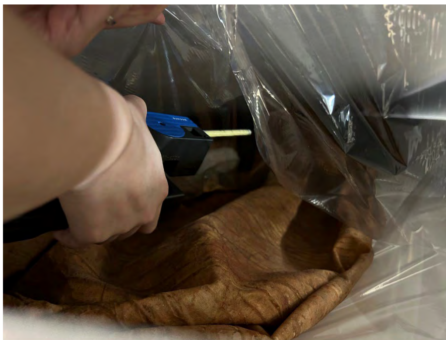
Figure 7: Testing for VOCs using the Drager pump in a mostly enclosed box the artwork was contained in.
