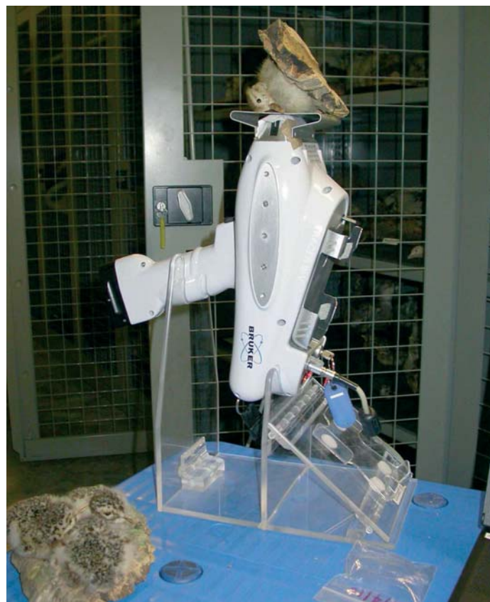
Testing for arsenic with the PXRF in a static position
