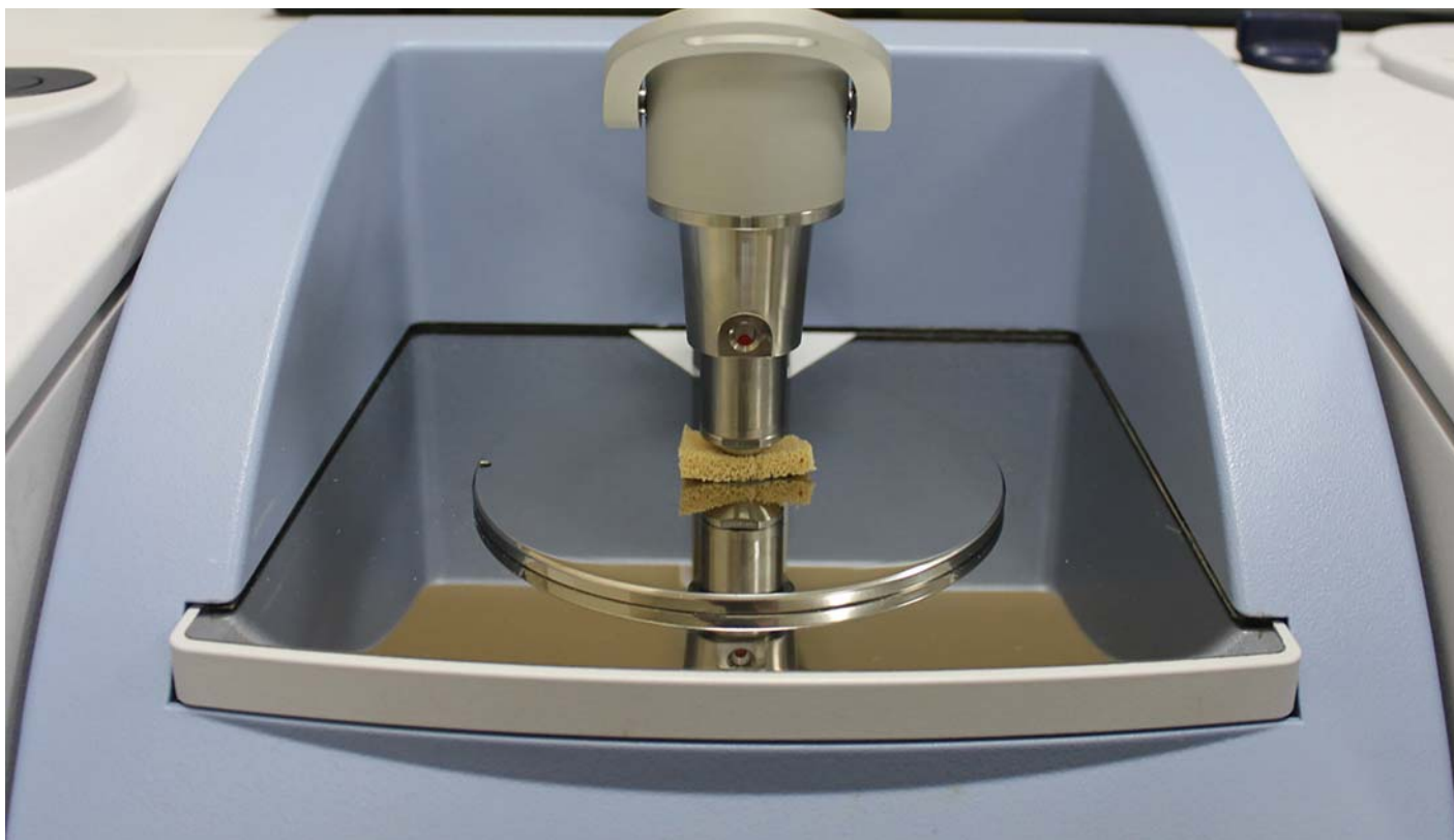
Attenuated total reflection infrared spectroscopy of a smoke sponge used for cleaning the embroidered banner
