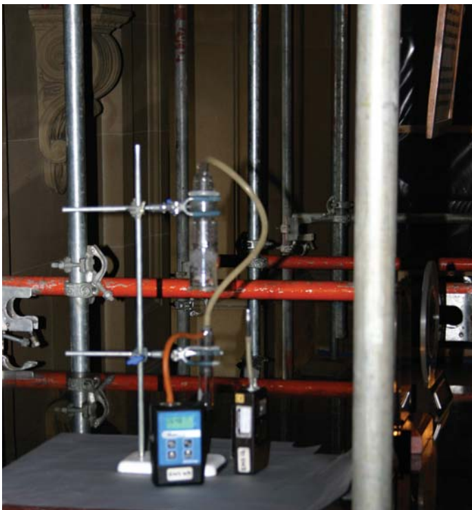
Testing for levels of ammonia gas
