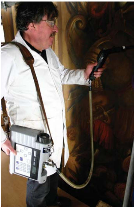
Testing for VOCs with a Toxic Vapour Analyser
