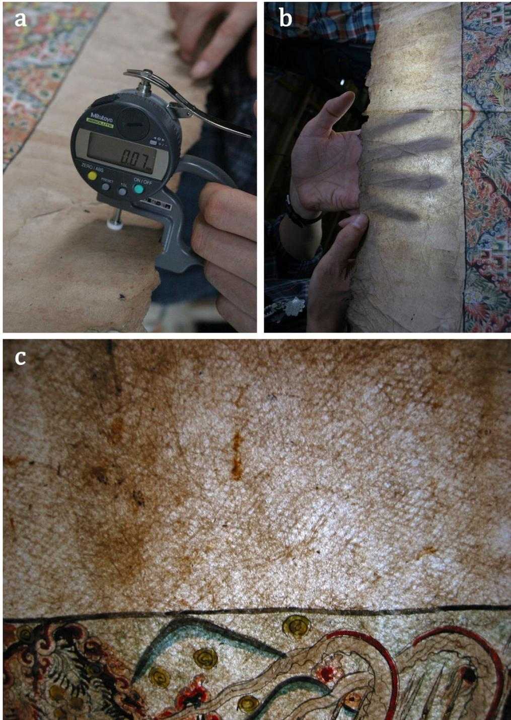
Figure 2. a) Measuring the thickness of *wayang beber*. b) Examining *wayang beber* using transmitted light. c) 1mm lattice beater mark pattern under transmitted light. © Sakamoto 2006.
