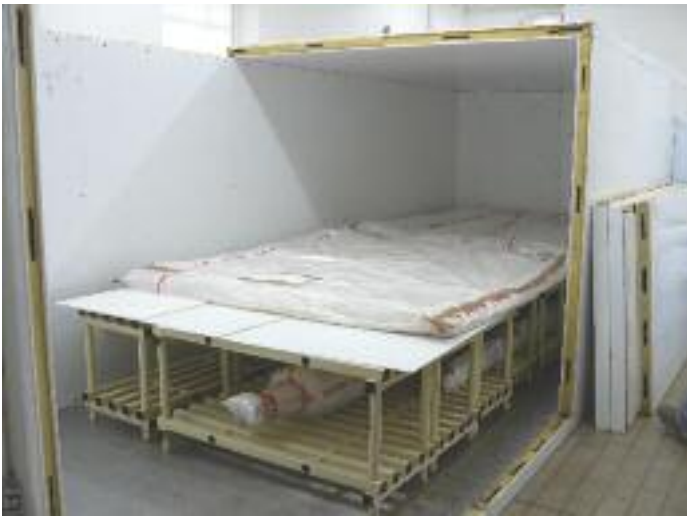
The freezer being built around the first mattress
