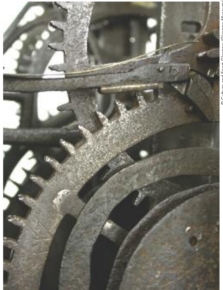
Detail of the 'nagshead' strike release
