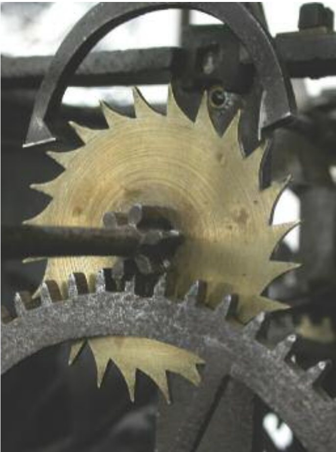
Detail of the anchor escapement with replacement pallet faces and wear in escape wheel
