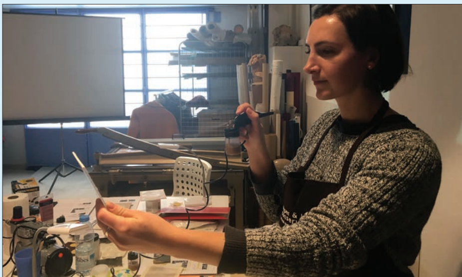
Jillian Gregory using an air compressor to create a very fine film of cellulose powder, which has previously been cooked to obtain some colour and can be used for colour matching repairs
