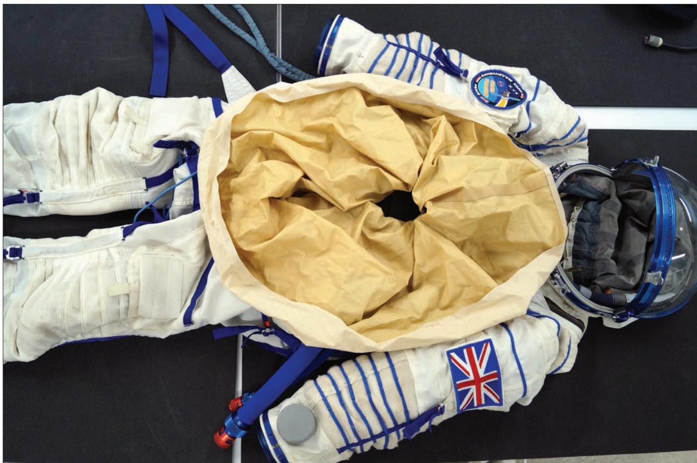
Sokol suit with chest opening visible. The fabric is gathered together and secured with a rubber band during spaceflight
