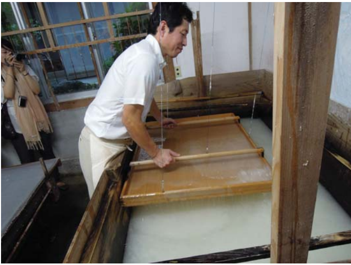
The papermaking studio in Mino. Forming the sheet from the paper pulp.
