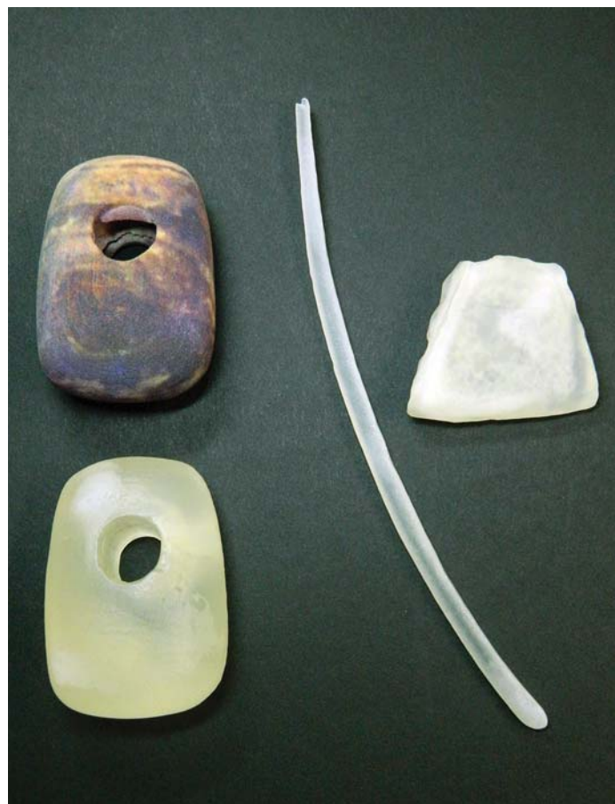
The 3D prints created with polymer jetting-based technology
