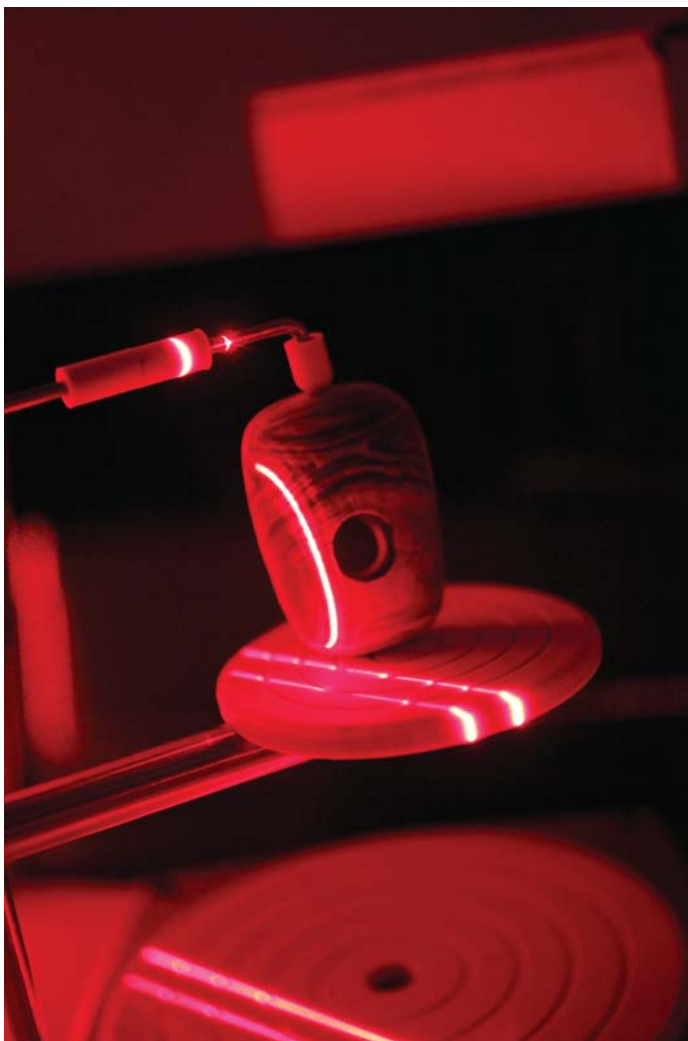
The original mace head specimen mounted and clamped for 3D scanning
