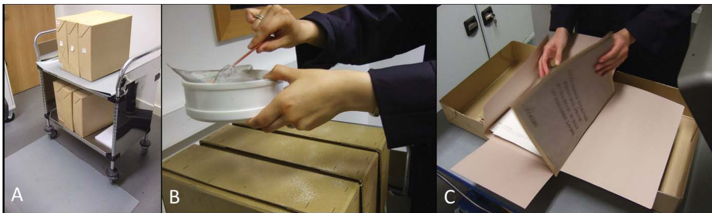
Boxes containing facsimile documents (A) were dusted with UV-fluorescing powder (B) before simulating standard handling procedures (C)
