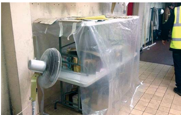
A wind tunnel used to dry wet books
