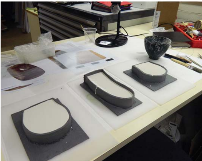
Using the 3D prints to create two piece silicon moulds with plaster supports
