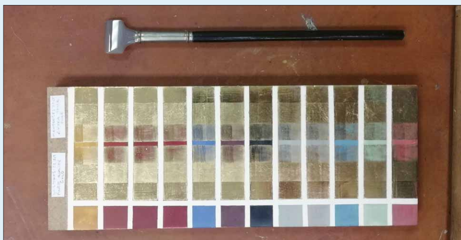
The reviewer's completed test panel with twelve colours and two types of gold leaf. Each sample has a burnished area, a matt area and a distressed area to show how each colour performs.
