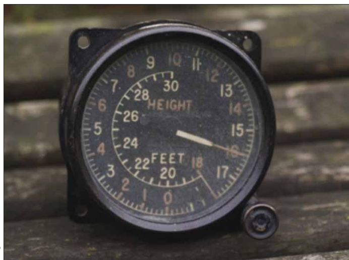
A radioluminescent altimeter from a WWII Spitfire
