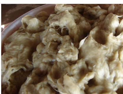
Fig. 14 *Kōzo* fibres after beating. Image copyright T. Kubo.
