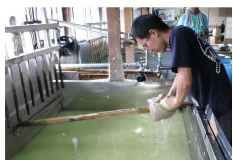
Fig. 15 Adding *tororo aoi* to the pulp solution in the vat (T. Kubo). Image copyright M. Mizumura.
