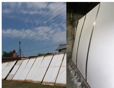
**Fig. 17** Drying: the wooden boards (left) and stainless steel wall (right). Image copyright T. Kubo.
