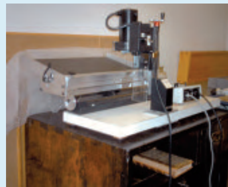
Board slotting machine at the Oxford Conservation Consortium
