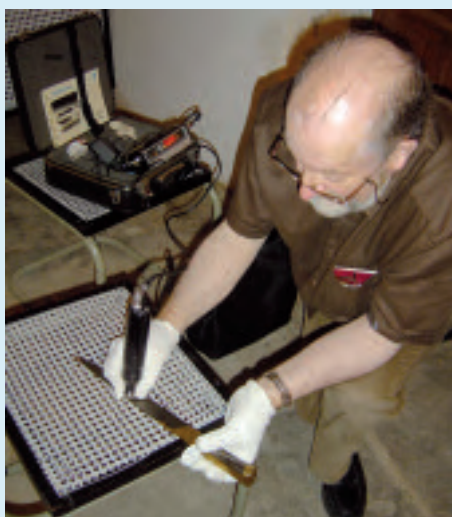
Archeometallurgist Dr. Alan Williams carrying out hardness tests
