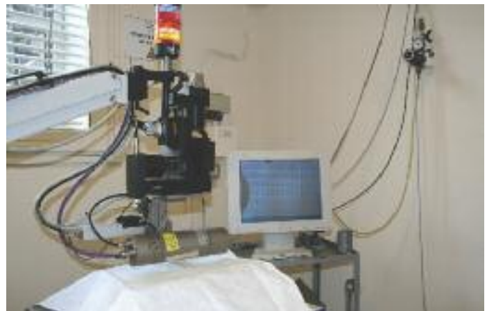
Fig. 4: XRF measurements were made using a Bruker Artax spectrometer fitted with a 1.5 mm collimator, operating at 50 kV and 0.8 mA, and counting for 200 seconds.
