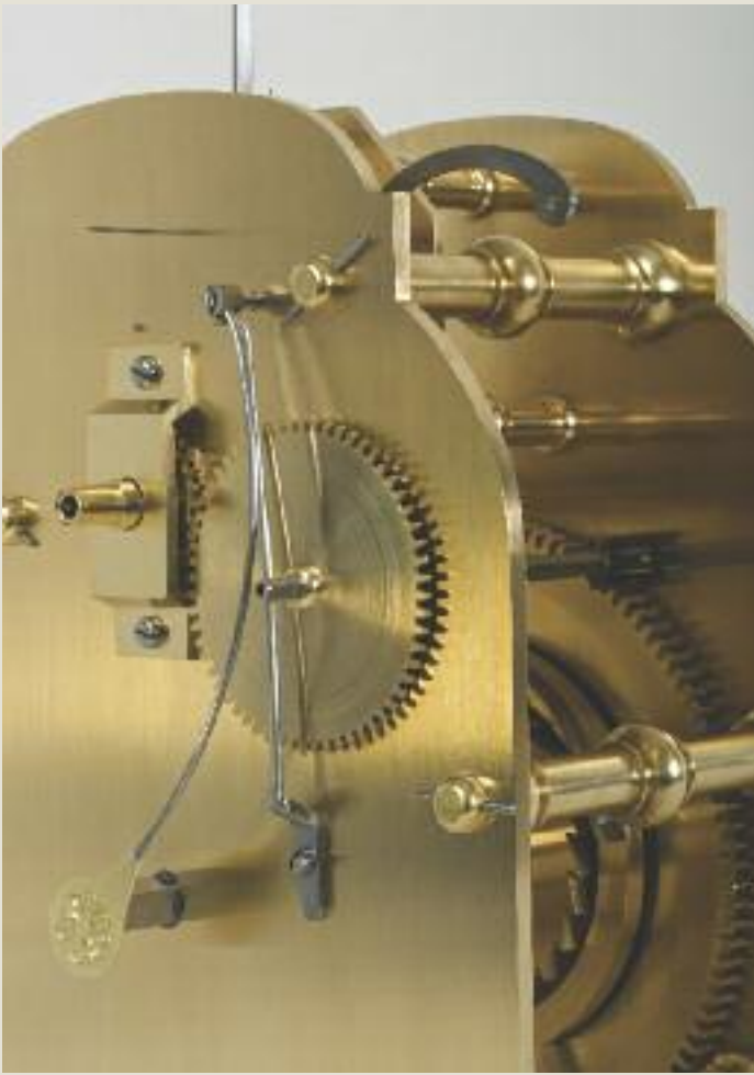
Bolt and shutter maintaining power is a safety mechanism that prevents the movement stopping whilst being wound. It is operated by pulling the lever (top right corner), which exposes the winding square.
