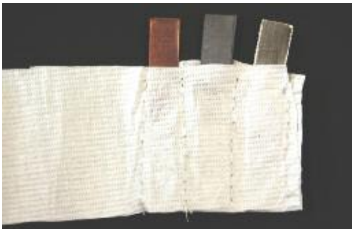
Fig.3: A 2g rectangle of Tyvek® was cut, folded in half and sewn with polyester thread to create pockets to hold the test coupons
