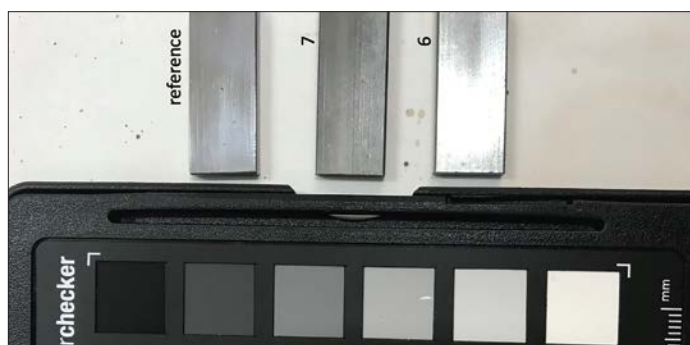
Steel strips at stage 2. Corrosion test after 1 month. 6 = Glycerin + Van Dyke Brown in DI; 7 = Glycerin + Van Dyke Brown in DI + dark soy sauce
