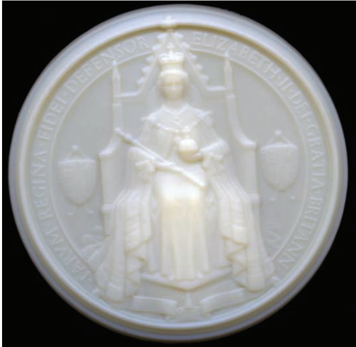
The replica seal in its original appearance after printing as a solidblock.
