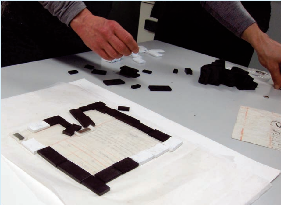
Drying a parchment sample under tension with magnets
