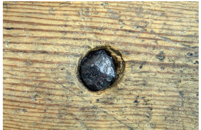
The underside of the base before and after treatment showing one of the nails holding the base together. The surrounding wood was cleaned, the corrosion on the nail was reduced and the nail then waxed
