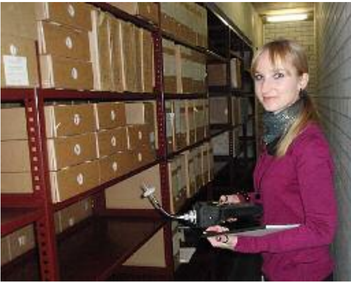
A student measuring the concentration of volatile organic compounds at the Nationaal Archief, The Hague
