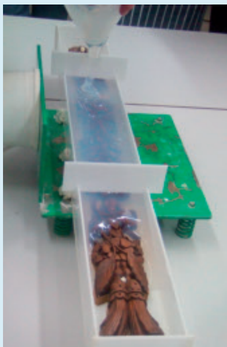
Pouring Silastic T4 into a prepared mould
