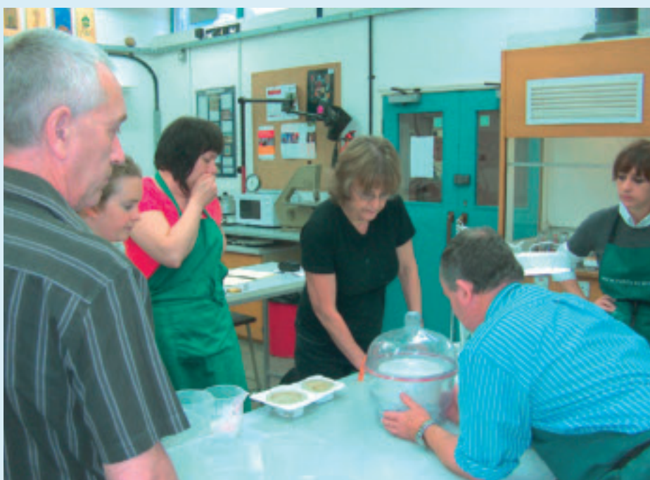
Campbell demonstrating the use of a dessicator and vacuum pump
