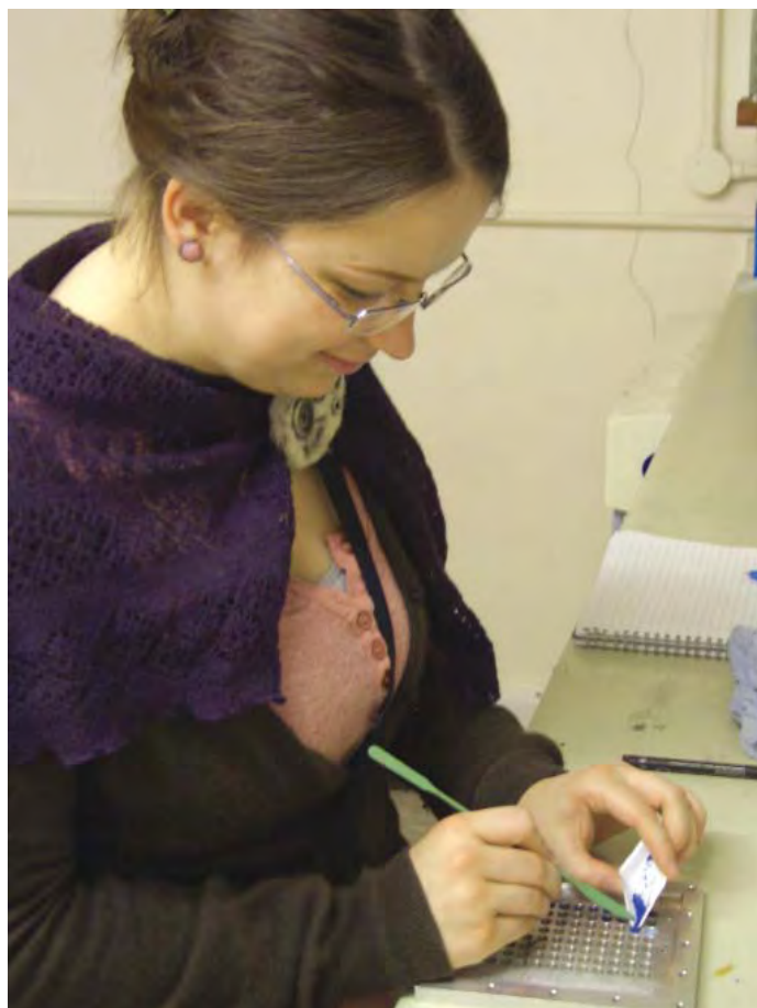
Helen puts sample into holder ready for the transmission scan
