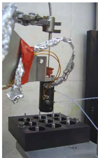
TEY set up: pigments in the holder below and detector clamped above
