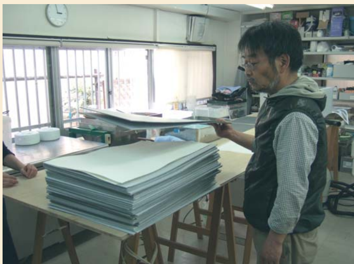
Mr Kibe prepares for the air-stream drying method – using corrugated cardboard to let air through.
