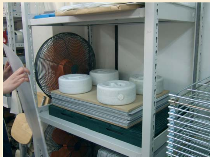
The air-stream drying chamber using a regular metal shelf unit and an electric fan – enables documents to dry in 1-3 hours without changing blotters.
