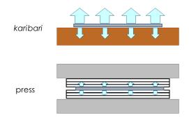
Fig. 1 Illustration of migration of water during drying. Light blue arrows mean water migration. Their sizes indicate speed of drying.
