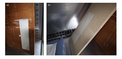
**Fig. 5** Photographs of samples, silk lined with paper, under *karibari* on (a) *karibari*-panel and (b) wood-panel.
