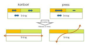
**Fig. 4** Influences of dimensional change of each part after moistening of assembled and lined objects. Blue arrows mean internal stress, and their size shows the strength of the stress. Brown arrows show the direction of change in formation.
