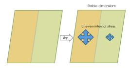
Fig. 3 Dimensional change and internal stress (blue cross arrows) during press-drying. Ideally, there is no dimensional change in this method.
