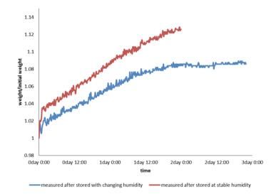
Fig. 6 Influences of conditions during *karibari* on changes in weight of samples which are exposed to high humidity (23  $^{\circ}$ C and 80% relative humidity).
