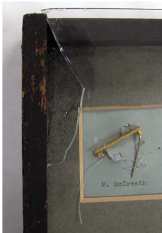
Fig.5. Glass broken along the edges in contact with the wood frame. As a result, shards settled in the cases and became intermingled with objects that had come free of the glue matrix
