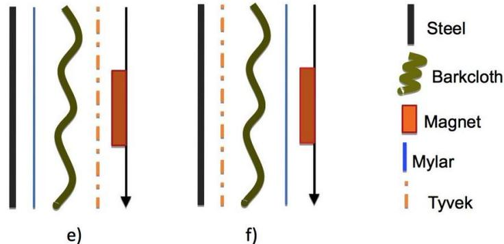
Figure 8. Barkcloth with both polyester film and polyethylene Tyvek® : e) polyester film between the steel and barkcloth and polyethylene between barkcloth and the nickel coating of the magnet; f) polyethylene between the steel and barkcloth and polyester film between the barkcloth and the nickel coating of the magnet. © Spicer.
