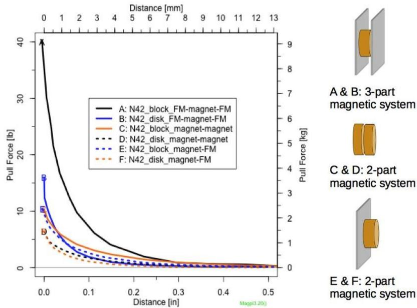
Figure 3. Field strength vs. distance relationships for two different shapes of magnets with the same grade: one block-shaped (N42, 1/2" x 1/2" x 1/8" thick) and another disc-shaped (N42, 1/2" diameter 1/8" thick) with another similarly sized magnet (C & D) or ferromagnetic material (E & F); or sandwiched between ferromagnetic materials (A & B). © Spicer, adapted from <https://www.kjmagnetics.com/calculator.asp>.
