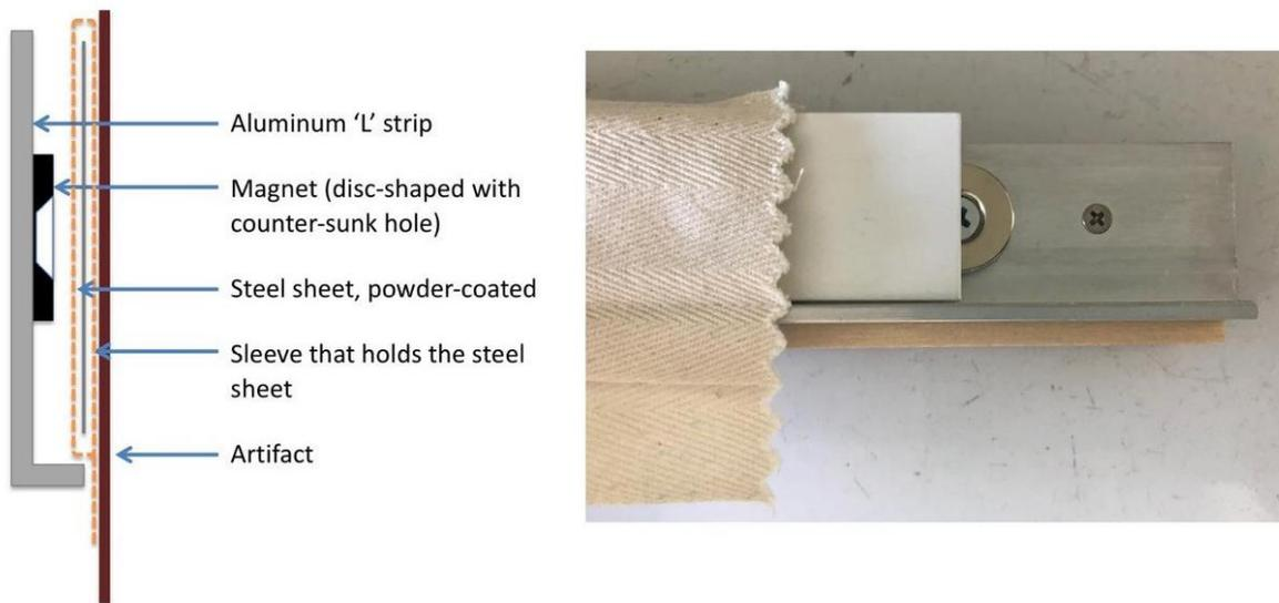
Figure 2. Cross section of the Mag Slat. The steel is inserted into a sleeve attached to the upper edge of the reverse-side of the artefact. The lower edge of the steel is supported by the lip of the aluminium 'L' and the counter-sunk disc-shape magnets keep the steel vertical. This is an example of large area pressure. © Spicer.
