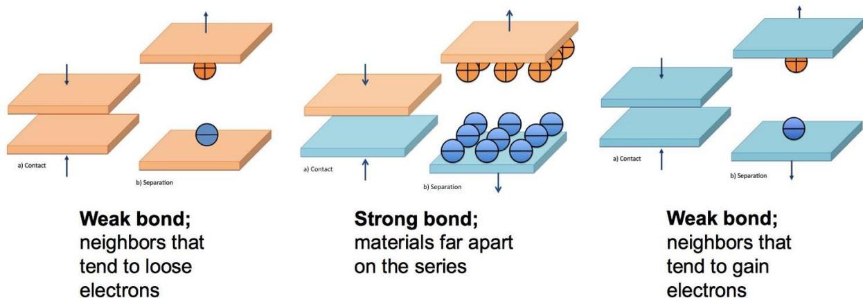
Figure 5. Schematic of electron exchange when two different materials are in contact and are then separated. The extent of this exchange and ability to create weak or strong bonds is based on the materials' placement on the triboelectric series, shown in Table 3. © Spicer.
