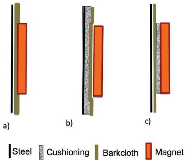
Figure 4. Schematic illustration of cushioning and lift: a) barkcloth being compressed within the magnetic system; b) barkcloth conforming to the magnet on a padded surface; c) barkcloth with cushioning below the magnet. © Spicer.
