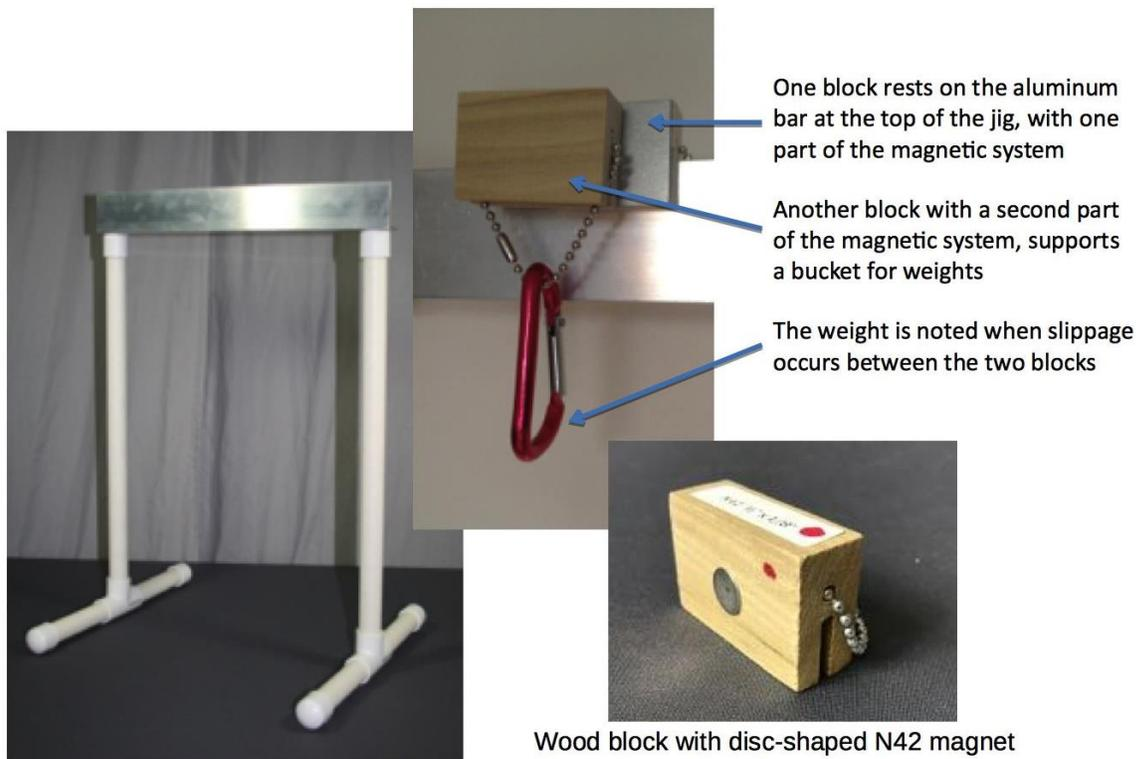
Figure 6. The jig set-up used for testing. A stationary block of 24-gauge steel is supported on the jig, while another block has a N42 disc-shape 1/2" x 1/8" neodymium magnet incorporated. © Spicer.
