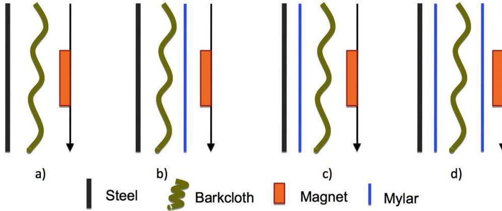
Figure 7. Four methods for layering materials within a magnetic system: a) barkcloth between steel and the nickel coated magnet; b) barkcloth next to steel and polyester film (Mylar®) next to the magnet; c) polyester film next to steel and barkcloth next to the magnet; and d) barkcloth sandwiched between two layers of polyester film. © Spicer.
