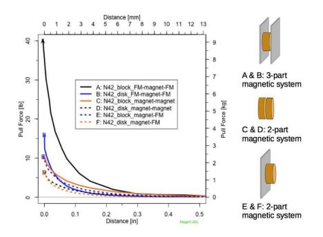
Figure 3. Field strength vs. distance relationships for two different shapes of magnets with the same grade: one block-shaped (N42, ½" x ½" x ½" thick) and another disc-shaped (N42, ½" diameter ½" thick) with another similarly sized magnet (C & D) or ferromagnetic material (E & F); or sandwiched between ferromagnetic materials (A & B). © Spicer, adapted from https://www.kjmagnetics.com/calculator.asp.
