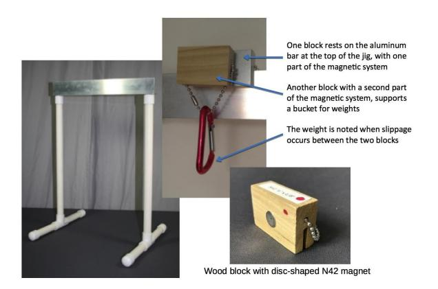
Figure 6. The jig set-up used for testing. A stationary block of 24-gauge steel is supported on the jig, while another block has a N42 disc-shape 1/2" x 1/18" neodymium magnet incorporated. © Spicer.
