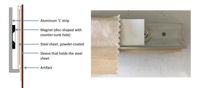
Figure 2. Cross section of the Mag Slat. The steel is inserted into a sleeve attached to the upper edge of the reverse-side of the artefact. The lower edge of the steel is supported by the lip of the aluminium 'L' and the counter-sunk disc-shape magnets keep the steel vertical. This is an example of large area pressure. © Spicer.
