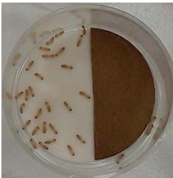
Figure 4 Example of experimental setup for testing the avoidance effect of plant extracts. One half of treated cellulose pad ( V. copallifera resin oil), dark brown in colour on one side on top of a moistened untreated cellulose pad covering the entire bottom of the dish (diameter approx. 45 mm, height approx. 35 mm). A total of 30 healthy termite workers ( C. formosanus ) were released for 24 hours and their position in the dish recorded.
