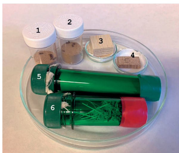
Figure 2 Insect samples on glass tray. 1: L. brunneus larvae inside the substrate, L. brunneus adults on substrate; 2: A. punctatum larvae inside substrate, A. punctatum adults on substrate; 3: A. punctatum eggs on oak wood; 4: L. brunneus eggs on oak wood; 5: Biotest tube with C. longicaudatum larvae and adults; 6: Biotest tube with clothes, T. bisselliella larvae and adults (© Nikolaus Wilke/ICM).
