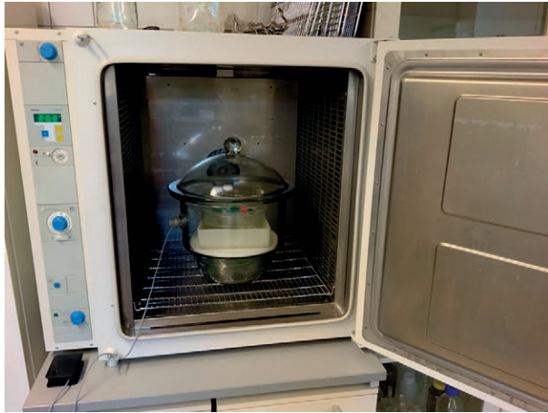
Figure 3 Heraeus UT 6200 heating test cabinet with desiccator containing the test samples. Note the cable of the temperature and humidity sensor on the left-hand side going into the desiccator (© Nikolaus Wilke/ICM).
