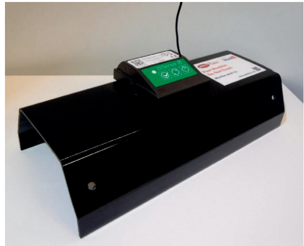
Figure 3 GTO detector mounted on drain guttering (© Chris Swindells/Kiwa 2021).
