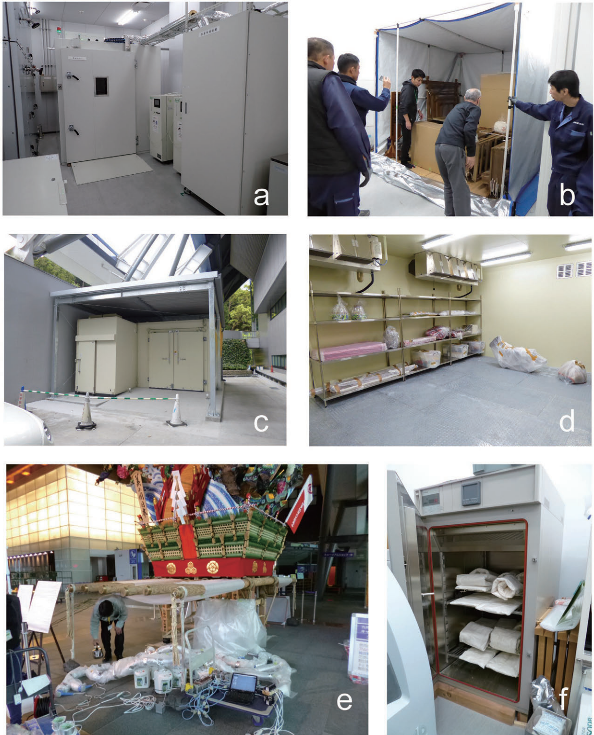
Figure 1 (a) Nitrogen treatment chamber; (b) CO 2 bubble; (c) walk-in freezer (−30 °C); (d) inside of walk-in freezer; (e) humidified warm air heat treatment (60 °C); (f) heat treatment (60 °C).
