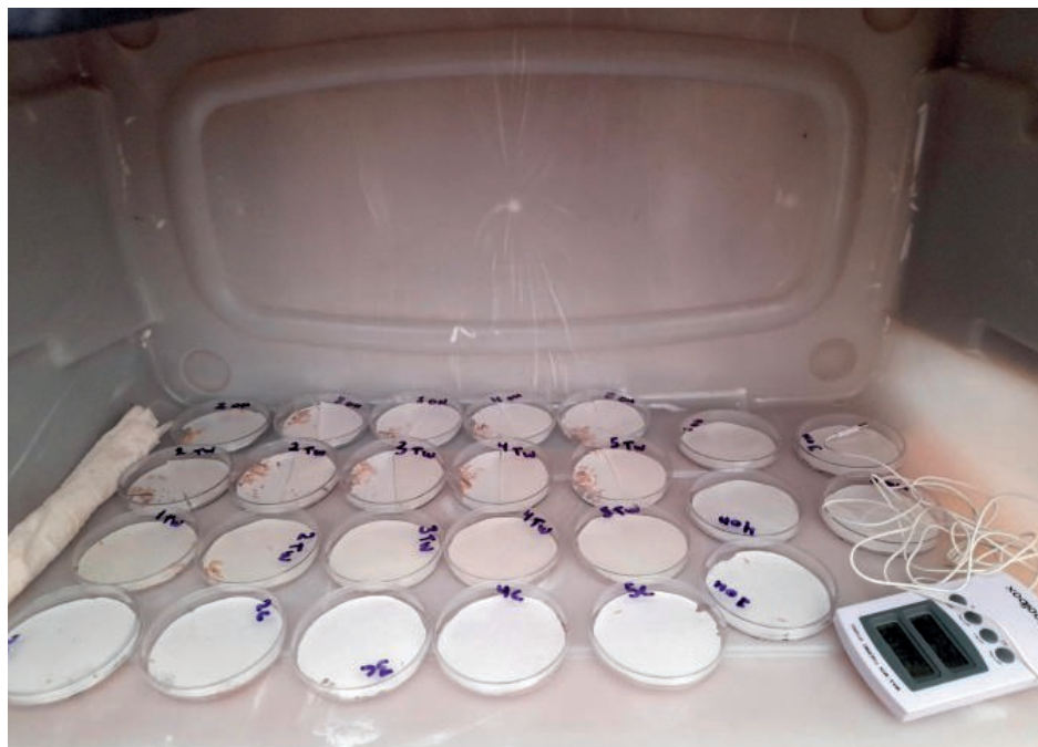
Figure 4 Setup for repellence and antifeedant tests on termites (© 2021 Eliana Quispitupac).
