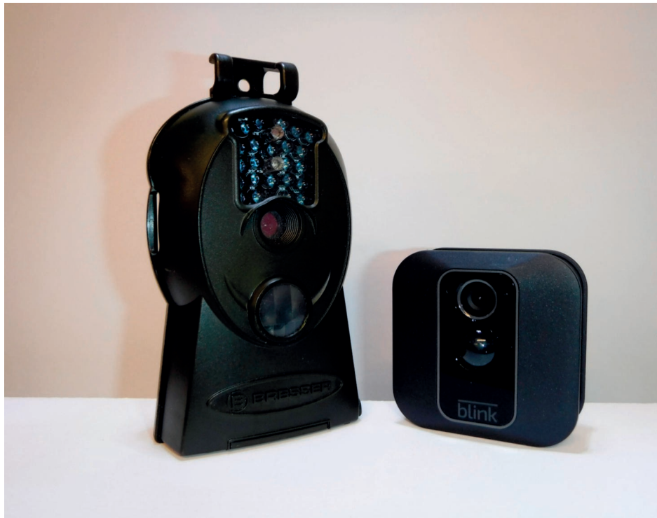
Figure 6 Examples of a dedicated trail camera and alternative home security camera which can be used to monitor rodent activity (© Chris Swindells/Kiwa 2021).
