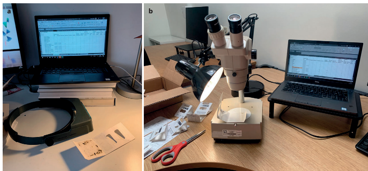
Figure 2 (a) Checking a blunder trap at home with 5× magnification optivisors, January 2021 (© Kristina Mandy). (b) Checking blunder traps with the right equipment at the NG, June 2021 (© The National Gallery, London).
