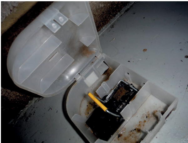
Figure 2 Example of 'intelligent' house mice exploiting the design of this protective box (© Chris Swindells/Kiwa 2021).
