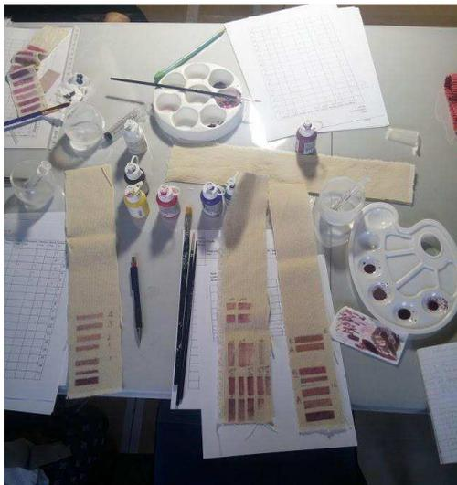
*Figure 2.* The conservators learnt how to make recipes using the drop-by-drop method of Lascaux's primary watercolour system.
