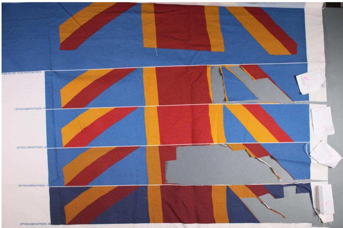
*Fig 7.* Printed samples used for Oddy testing *Table 4* © The British Library Board
