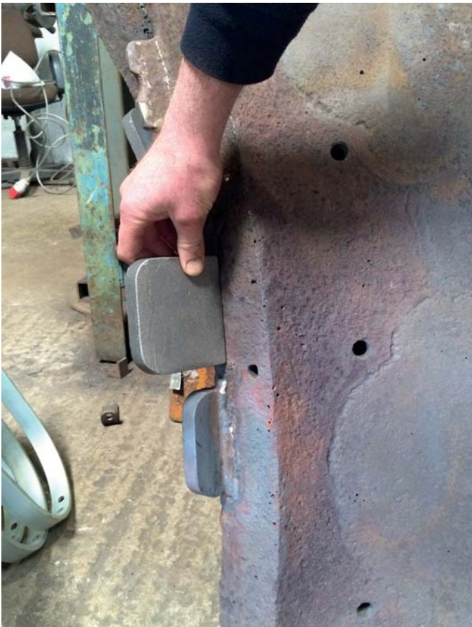
A replacement lug is placed in the fixing position
