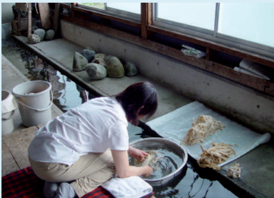
Washing the kozo fibers from impurities (Mino, Hasegawa Washi Kobo workshop)
