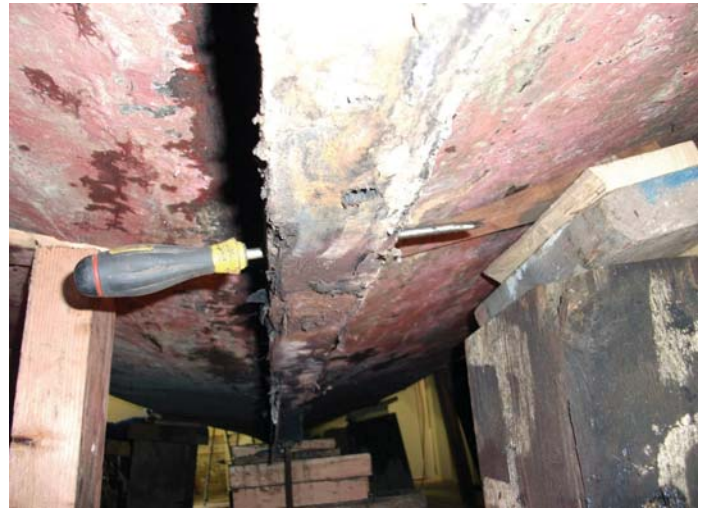
The state of the keel of Steam Pinnace 199
