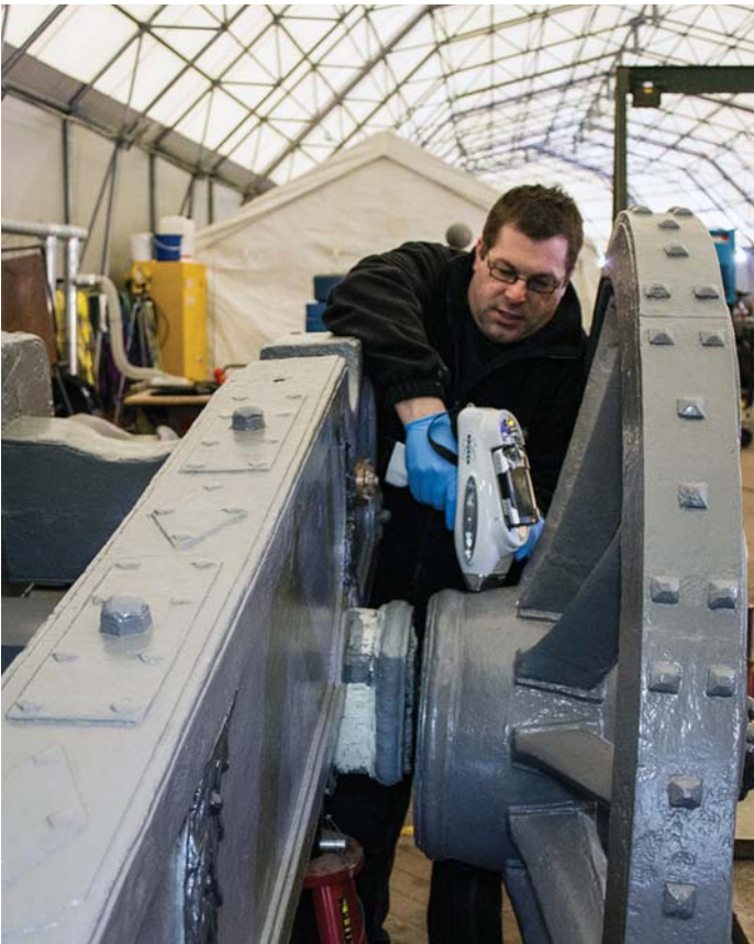
Using the XRF unit on a gun carriage in a conservation project for the Royal Artillery
