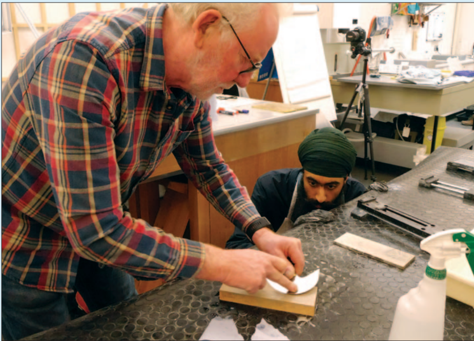
Bernard Allen demonstrating sharpening a curved blade on a Japanese whetstone
