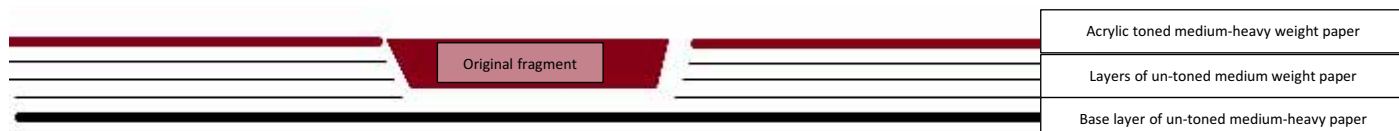
A diagram showing the layers of paper used in the infill
