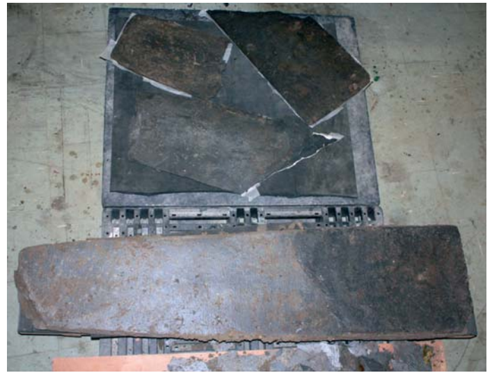
Removed surface fragments and lower layers after dry brush-cleaning
