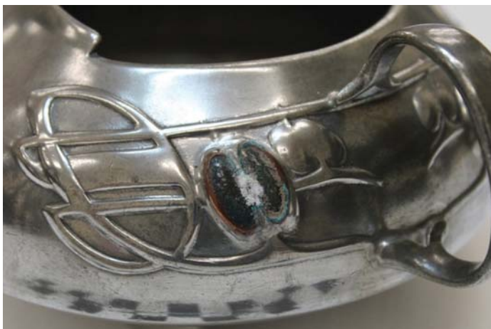
Milk jug showing a loss of enamel and white crystalline material
