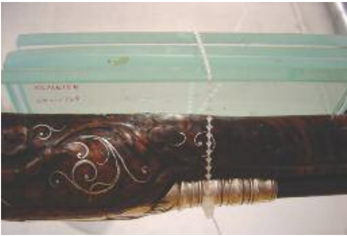
Glass weights being used to hold the two-halves of the forestock in the correct alignment
