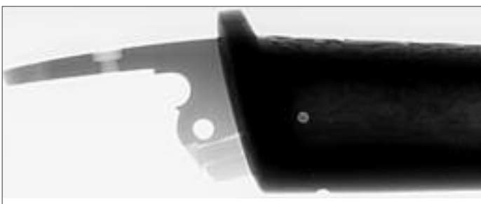
X-ray showing how tang attached, 280kV, 5mA, 30 sec
