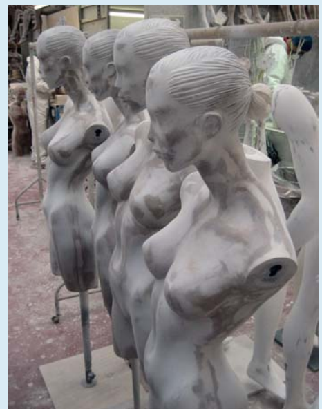
Fibreglass forms after sanding
