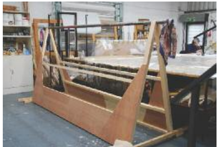
Figure 6: The transportation structure (note that the cardboard tube is missing from the image; it was threaded around the central steel pole before the painting was draped across)
