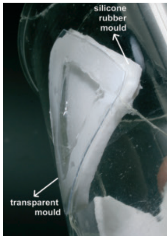
Fig 1 The mould: silicone rubber inside & PVC transparent sheet outside.
