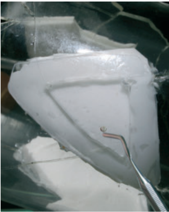
Fig 8 Tapping on the plastic mould with a metal spatula to help an air bubble to rise towards the air hole
