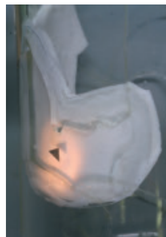
Fig 6 An illuminated mould: a shadow thrown by the triangle on the mould's inner wall made of silicone rubber is clearly visible
