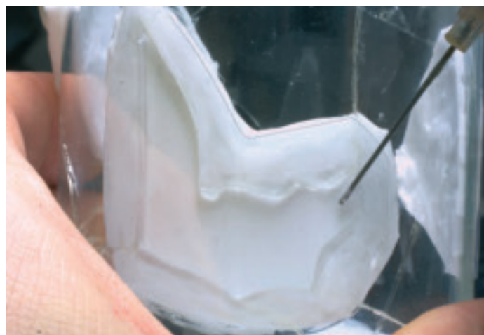
Figs 7 Injecting epoxy resin by means of a needle penetrating the mould.
