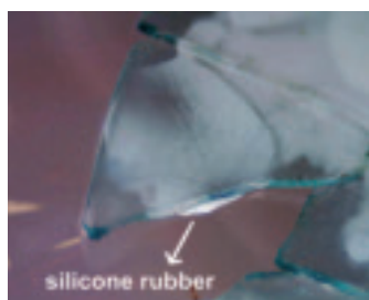
Fig 3 Silicone resin used to secure the mould has flowed into the mould
