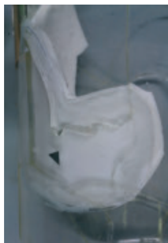
Fig 5 A triangle made of non-transparent material (aluminium foil) glued to the outer transparent mould
