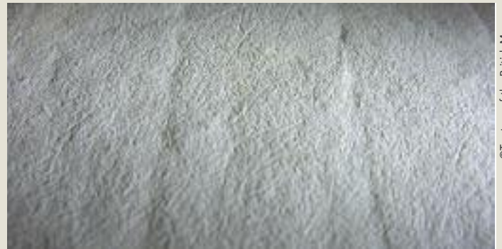
Raking light detail revealing impressions from the rough felt used for pressing and unusually deep chain lines
