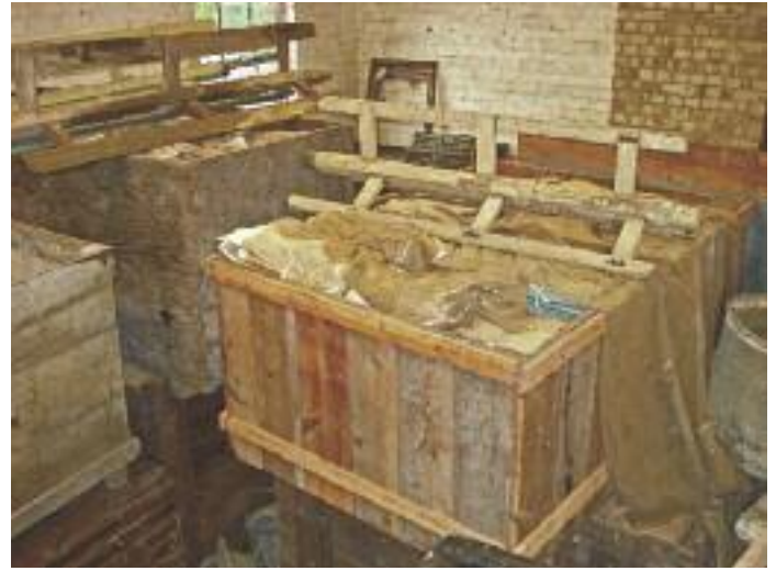
The 1930s to 1950s correspondence in open crates. The 3 bladed wooden stirrers were used to agitate pulp in the papermaking vats
